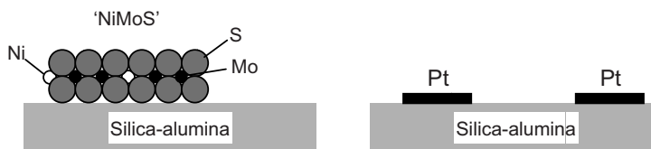
Figure 3.31 Models of hydrocracking catalysts; left: \text{NiS}/\text{MoS}_2/\text{silica-alumina} ; right: \text{Pt}/\text{amorphous silica-alumina} .
